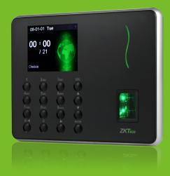
WL10 is Fingerprint Time & Attendance Terminal with Wi-Fi module. With Wi-Fi function, User needn't wire Ethernet cable, it supports hotspot mode and allow mobile APPs connection and check in/out and download record directly. It's associated with ZK new fingerprint reader, the operation remains stable under strong light source and high preciseness of verification of wet and rough fingers. It also has elegant design and slim sharp, it will start new stage of time attendance.
