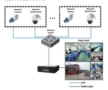
**Note:** The /H and /H/I models provide 12 HDMI outputs for video wall display.
